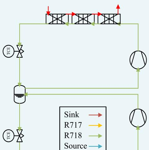
Intermediate pressures and temperatures are optimised for highest COP.
